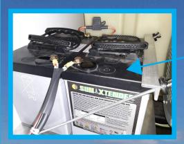
2 Premium Cycle on board batteries for 24 hour operation without generator
